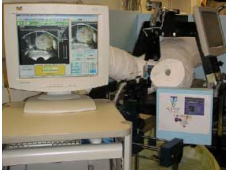
Figure 2: System for ultrasound-guided robotic brachytherapy (JHU & Burdette Medical)
