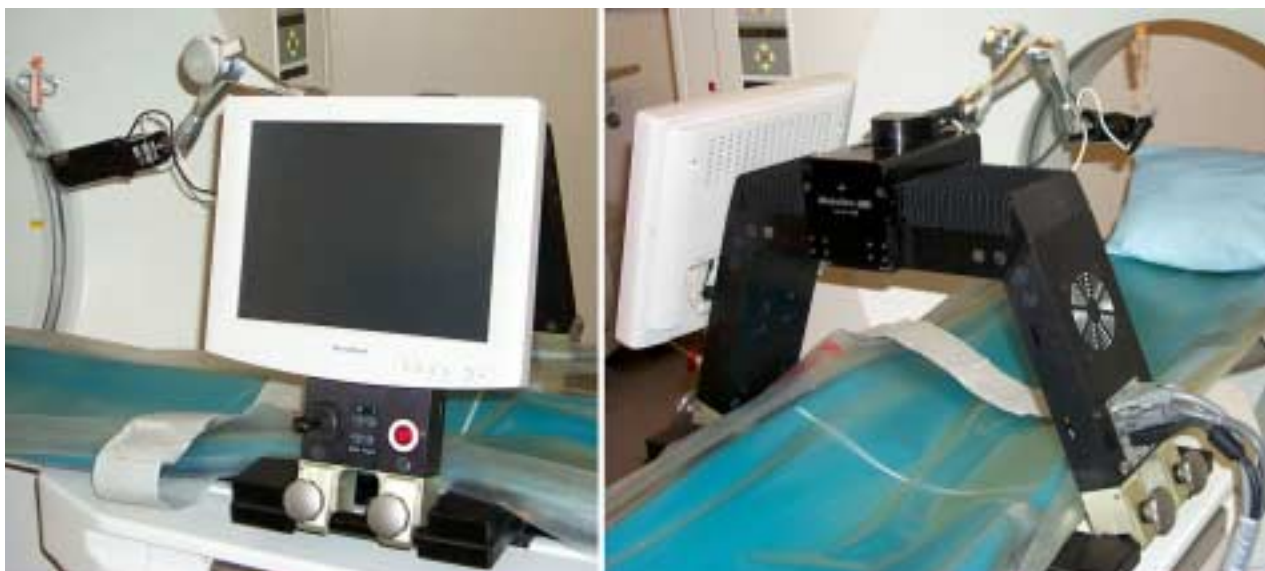
Figure 1: Tracker robot for CT guided interventions, URobotics, JHMI
