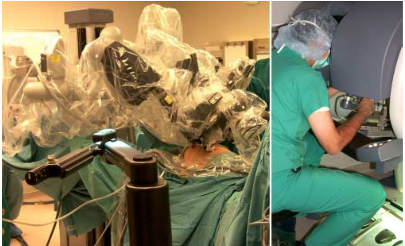
Figure 3: AESOP arm (foreground - left) and daVinci system (background - left, and surgeon's console - right) in a laparoscopic prostatectomy case at JHMI
