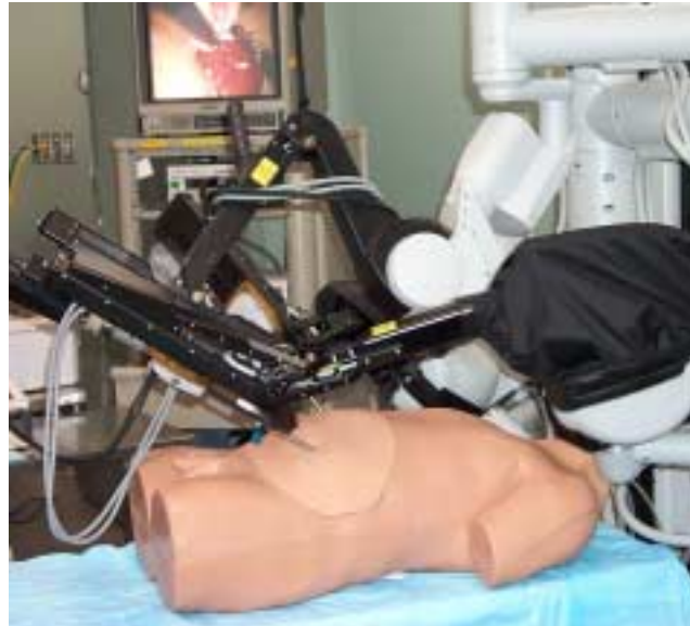
Figure 5: High-Fidelity synthetic torso for urologic laparoscopy training (URobotics, JHMI)
