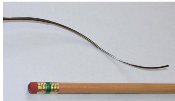
Fig. 1: An active cannula consisting of three concentric, telescoping, precurved Nitinol tubes. Cannula shape can be controlled by rotating and translating the tubes at their bases.
