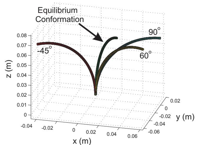
Fig. 4. The equilibrium conformation of three identical tubes, rotated to  $60^\circ$ ,  $90^\circ$ , and  $-45^\circ$  is shown to be non-planar. All three tubes must undergo both bending and torsion in order to reach this configuration.
