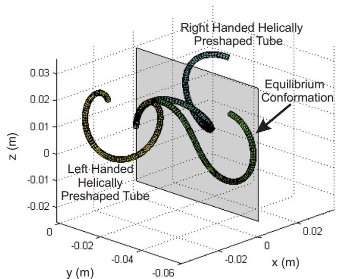
Fig. 7. Another possible equilibrium conformation of two helically shaped tubes with equal stiffnesses.
