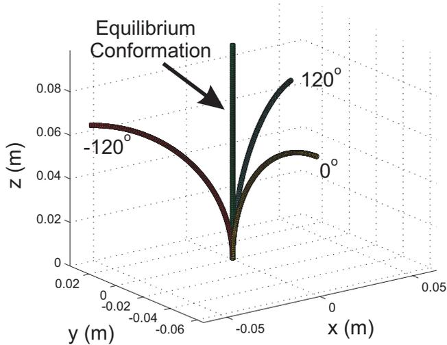
Fig. 2. The equilibrium conformation of three identical circular tubes spaced evenly at  $0^\circ$ ,  $120^\circ$ , and  $-120^\circ$  is straight
