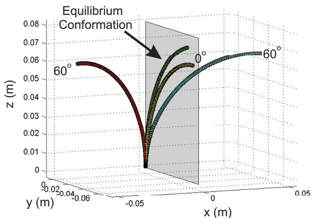
Fig. 3. The equilibrium conformation of three identical tubes rotated to  $0^\circ$ ,  $60^\circ$ , and  $-60^\circ$  lies in the plane of symmetry at  $0^\circ$ .
