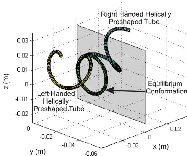
Fig. 6. One possible equilibrium conformation of two helically shaped tubes with equal stiffnesses.
