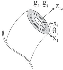
Fig. 2. The coordinate frames for the first and the  $i$ th tubes at an arbitrary cross section of the active cannula. They differ by an angular rotation of  $\theta$  about their  $z$ -axes, which are both tangent to the curve. The curvatures,  $\omega$  and  $\omega_i$ , of the frames are not pictured, since they may in general lie in any direction with respect to the coordinate frames.
