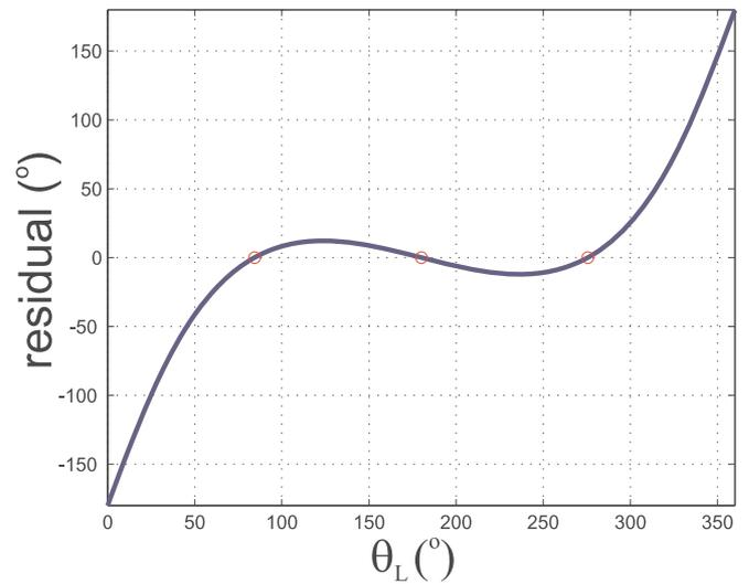
Fig. 4. Plot of the left-hand side of Equation (43) versus  $\theta_L$  for the tubes in Table 1 and  $\theta_0 = 180^\circ$ . Solutions for  $\theta_L$  satisfying (43) are shown at  $\theta_L = 180^\circ$ ,  $\theta_L = 84.4^\circ$ , and  $\theta_L = 275.6^\circ$ .
