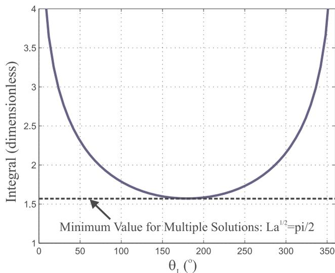
Fig. 5. For  $\theta_0 = 180^\circ$  the value of the integral in (44) is shown in blue as a function of  $\theta_L$  ranging from  $0^\circ$  to  $360^\circ$ . Because it is lower bounded by  $\pi/2$ , the dimensionless parameter  $L\sqrt{a}$  can be used to predict when multiple solutions can occur.
