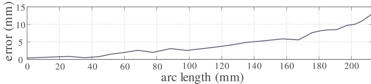
Fig. 12. Error versus arc length for the 200° partial overlap case with nominal parameter values using the model of Section 4. The general increase in error from base to tip is characteristic of all experiments, and thus tip error provides a reasonable metric for our experimental dataset.
