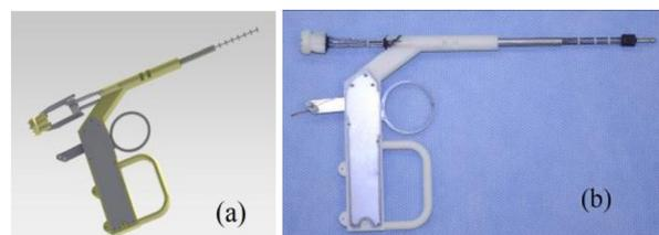
**Fig. 2 (a) CAD model of tool design, and (b) prototype of tool**
