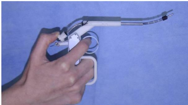
**Fig. 4 Prototype deflecting upward under hand control**
