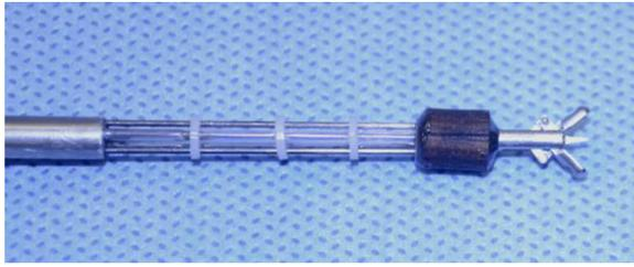
**Fig. 3 Multi-backbone bending mechanism with grasper**
