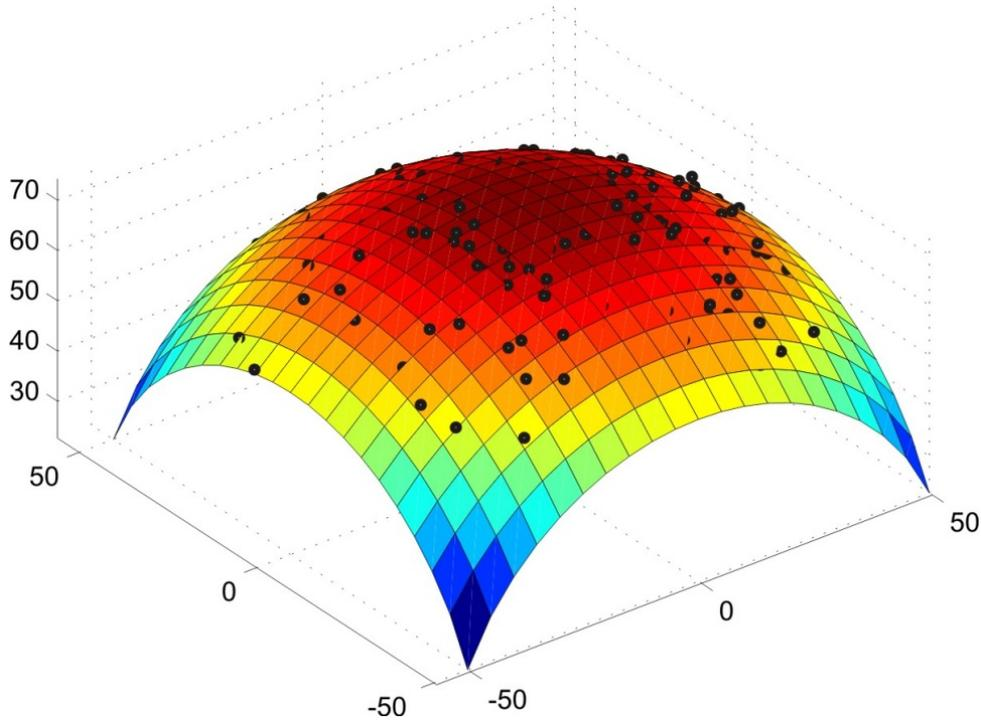
**Figure 8.** When used to scan a plastic sphere, the conoscope returns a point cloud (black dots above) which can be used to align preoperative image information (here represented by the spherical surface) with this “intraoperative” point cloud.
