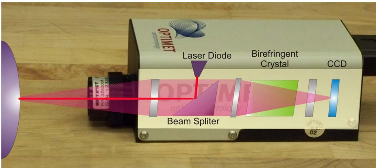
**Figure 1.** A photograph of the Optimet Conoprobe Mark 3.0, the off-the-shelf conoscopic holography system used in our experiments, which provides highly precise 1D distance measurements. Superimposed is a conceptual diagram of the basic components generally used in conoscopic holography, which process the returned light. The end product is an interference fringe pattern on the CCD sensing array at the back of the device, from which distances are computed.
