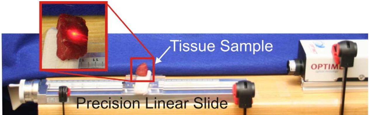
**Figure 4.** Baseline conoscope measurements were collected using a manually actuated precision linear slide. Tick marks on the actuation handle (visible at the left-hand end side of the slide above) can resolve 10 micrometers of linear sample motion. One full handle revolution produces 2mm of sample travel.
