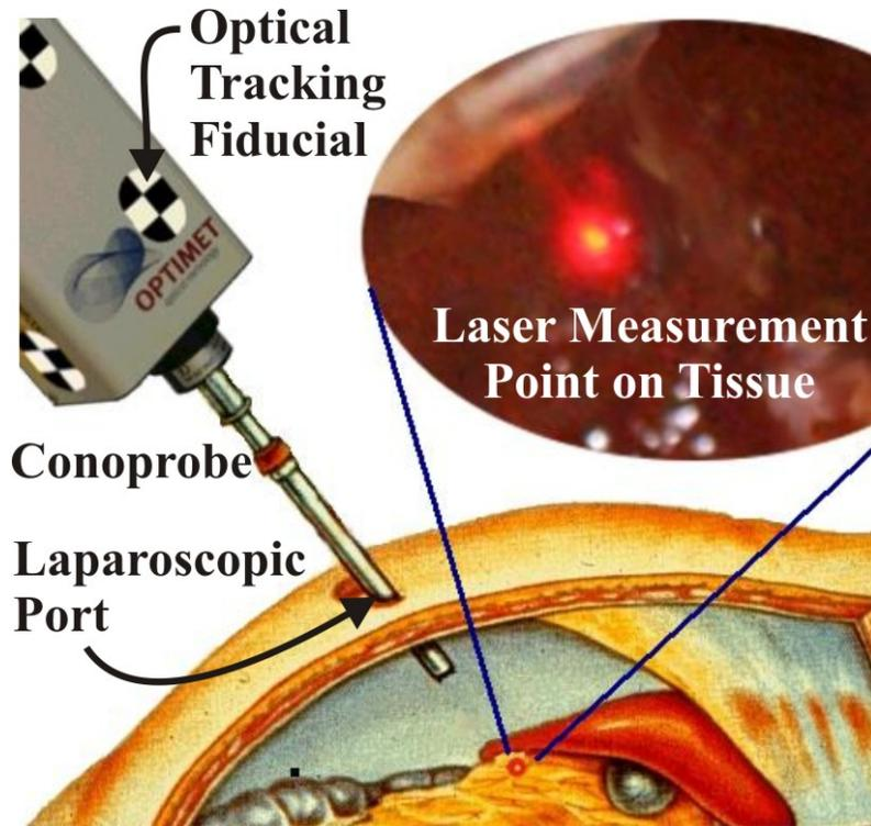
**Figure 2.** Conceptual drawing of organ surface scanning using conoscopic holography. The tracked conoscope returns distance measurements, which are converted to a point cloud that defines the shape of the tissue surface.
