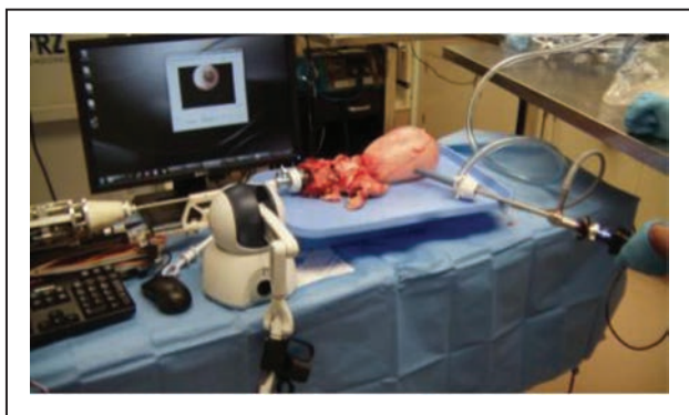
FIGURE 3. Overview of ex-vivo bovine bladder experimental set-up. Screen shows endoscopic robot view. Transvesical laparoscope used for procedure monitoring and capture of images. The figure shows the slave robot's actuation unit and the master manipulator (Sensible Phantom Omni) along with endoscopic view on screen in background. Reproduced with permission from [15**].
