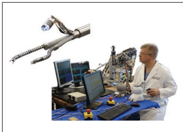
FIGURE 6. The phase I in-vivo single port access system shown in a deployed state with two 7 Degrees of Freedom dexterous arms and a controllable stereovision camera head. Original figure from Simaan and Herrell.
