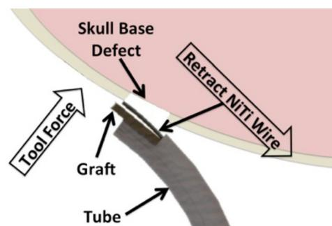
Fig. 2 Shelved tube with NiTi wire gripping design
