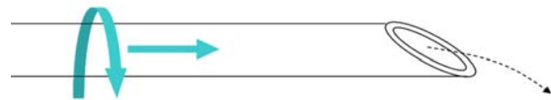
Figure 1: When a bevel tipped needle is inserted into tissue, asymmetric tip forces cause it to bend in a curved path as it cuts through the tissue. Correction for error and obstacle avoidance can be achieved by controlling axial rotation at the needle base during insertion.
