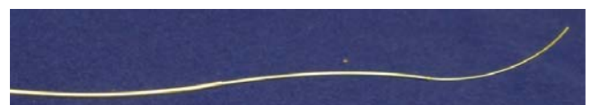
Figure 2: An active cannula composed of 3 concentric pre-curved nitinol tubes. The shape of the device can be changed by the relative rotation and translation of component tubes at their respective bases.
