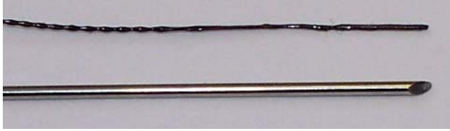
Figure 4: Bevel tipped needle with magnetic tracking coil
