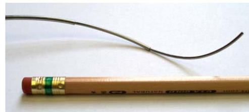
Fig. 1. Picture of an active cannula, a miniature surgical continuum robot actuated by the translation and rotation of concentric precurved tubes.
