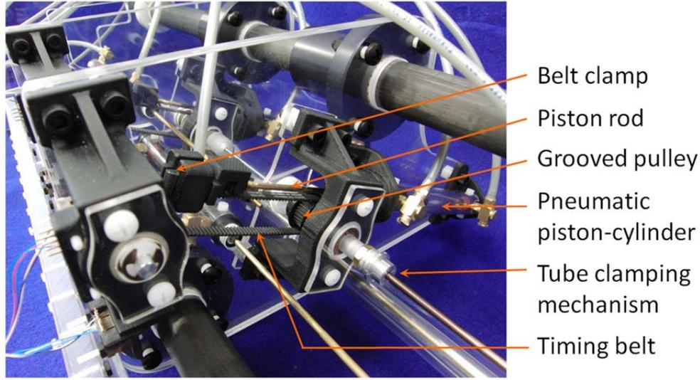
**Figure 4: Transmission for rotary motion of needle tube**
