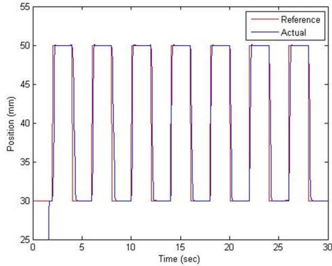
**Figure 5: Position tracking for translation of sliding plate**
