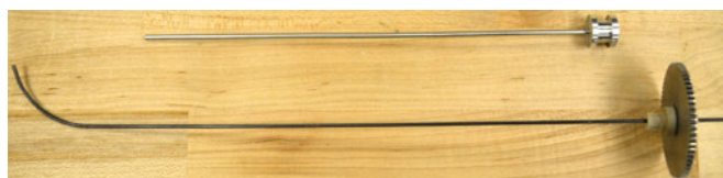
Fig. 5. Tubes are permanently attached to hubs using a biocompatible glue and can be autoclaved. The precurved aspiration tube has an additional gear attached to the hub to rotate the tube.
