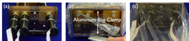
Fig. 3. Sterile barrier concept. (a) Motor plate is removed from the robot before sterilization. (b) Sterile bag is attached to the sterile robot using an aluminum bag clamp, enabling the motor plate to be subsequently attached and the motors to engage with the Oldham couplings (see Fig. 4). (c) Motor plate is reattached and the bag pulled over it. The robot is now sterile.
