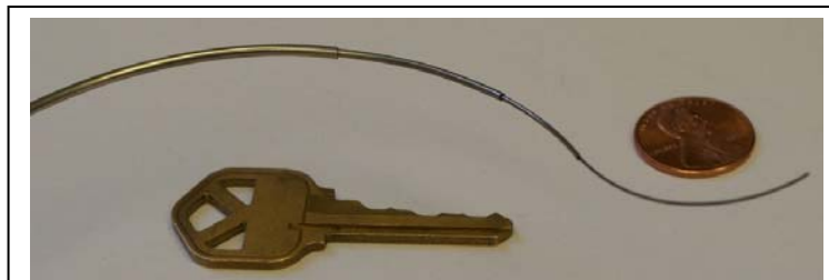
Figure 2. A prototype 4-tube Active Cannula (AC), made from precurved superelastic tubes, which changes shape as tubes are extended and rotated relative to one another. The USITT shown in Figure 1 was integrated with the AC to create the ACUSITT steerable acoustic ablator – the first steerable needle with an integrated interventional tool of which the authors are aware.
