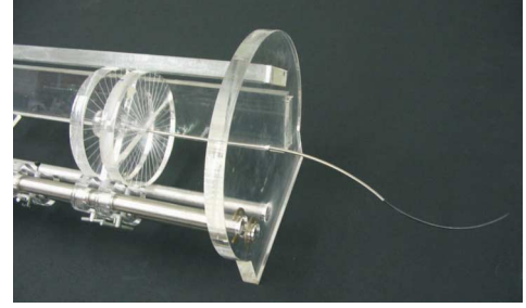
Fig. 9. Manual actuation mechanism. Both tube and wire have input circular handles etched to encode rotation and the support structure features a linear ruler etched to encode translation. Spring pin locking mechanisms hold the wheels at desired linear and angular positions.
