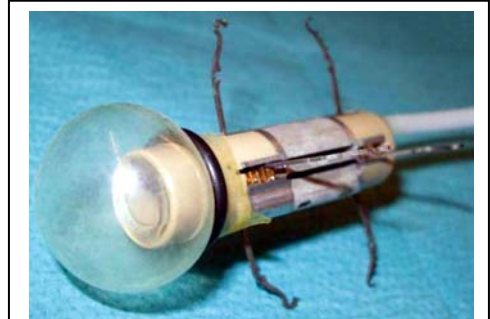
Figure 1. Legged capsule robot from prior work, showing tether inflated frontal balloon, which houses a wireless CCD camera. Image courtesy of the CRIM Lab SSSA, Italy.
