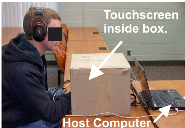
Figure 3: A user interacting with the touchscreen during the user studies. The user was able to touch the screen, but not view it, and the user's ears were shielded to prevent auditory feedback from touchscreen actuators during haptic experiments.
