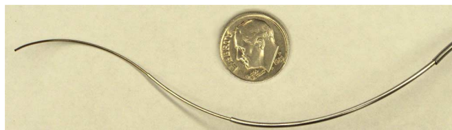
Fig. 1. Prototype active cannula made of three superelastic nitinol tubes and one central wire.
