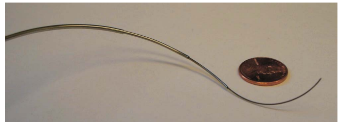
Fig. 1. A prototype active cannula made of superelastic nitinol tubes. Four tubes are shown in the figure above, ranging in diameter from 1.8 mm to 0.5 mm which can rotate and translate with respect to each other to change the cannula’s shape.
