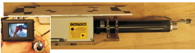
Fig. 13. First prototype of a laparoscopic tube attached to the Conoprobe. A small CCD camera is attached to the tip of the tube, enabling the physician to view the position of the laser measurement spot on a handheld display screen. (Inset, lower left) Display screen and the tip of the tube seen end-on. This first prototype illustrates the basic concept, but is not yet airtight.
