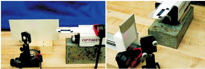
Fig. 7. Experimental setup for mirror deflection experiments (left) rotating mirror experiment and (right) fixed mirror, translating sample experiment.
