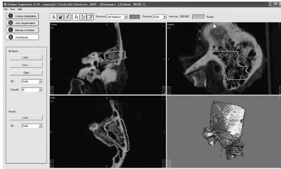
FIG. 3. Screenshot of the software used for the segmentation. The surgeon contours the region to drill in the axial view of the image ( bottom left ). A three-dimensional shape of the region chosen for milling is displayed to the surgeon at the end of the segmentation.
