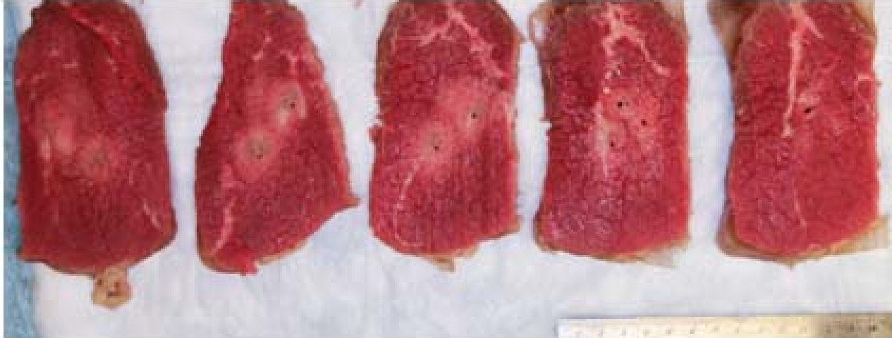
Figure 9. Slices of Bovine muscle tissue that was ablated using the ACUSITT. These experiments were carried out using the experimental apparatus shown in Figure 4(Left), and demonstrate deployment to successive locations through a single tissue puncture point, in a spatial pattern similar to that shown in Figures 6 and 7. Slices containing one, two, and three ablations are shown.
