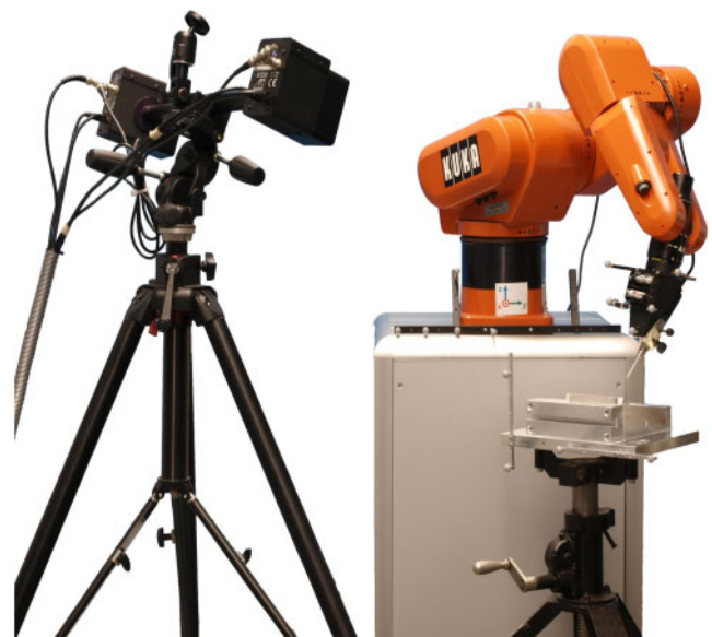
Fig. 1 The robotic system at Hannover with the KUKA KR 3 , the ARTTrack2 , and the mounting device
