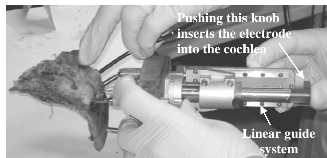
Figure 3. Insertion tool attached to the temporal bone specimen via Microtable to guide the electrode array into the cochlea through the drilled path.
